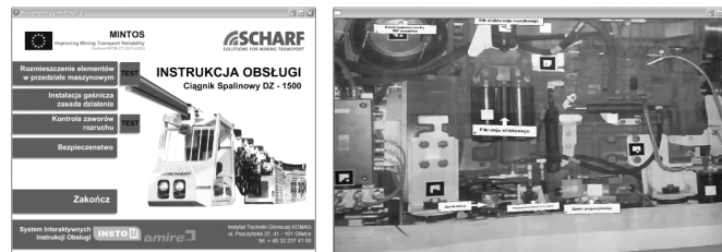
Fig.5. Arrangement of diesel engine systems in machinery compartment – training programme realized with use of Augmented Reality technology
