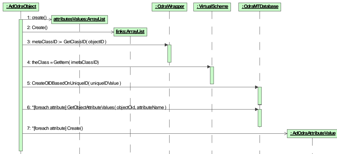
Figure 74. Sequence diagram for creating an object – part (a).
